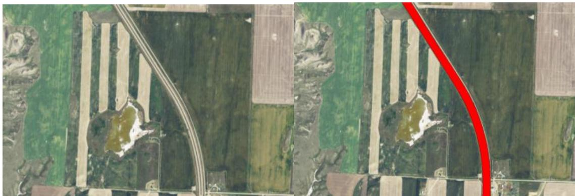
Figure 7- NAIP imagery and an Interstate route sampling location. Montana DOT Vegetation layer off (left) and on (right). Layer ROW boundaries match fence lines and transition from prairie grassland to cultivated cropland outside ROW boundary.
