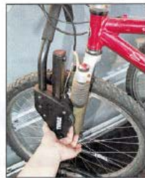
4. Slide rack down firmly on front tire.
