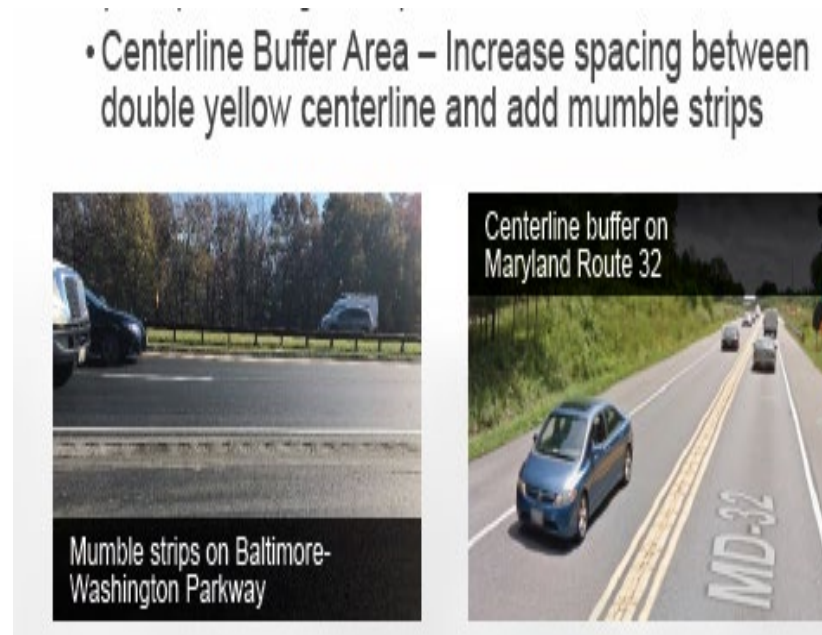
Figure 197: Centerline Buffer Area (Street views from Google Maps)
