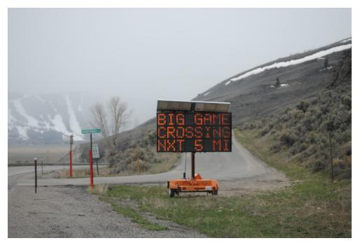
Figure 1. Variable message sign on highway skirting the National Elk Refuge in Wyoming. Credit: Rob Ament.
