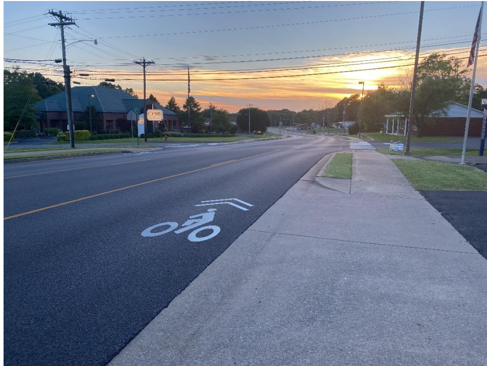
Figure 5: Shared lane use markings along E. Fifth Avenue in Calvert City, Kentucky.
