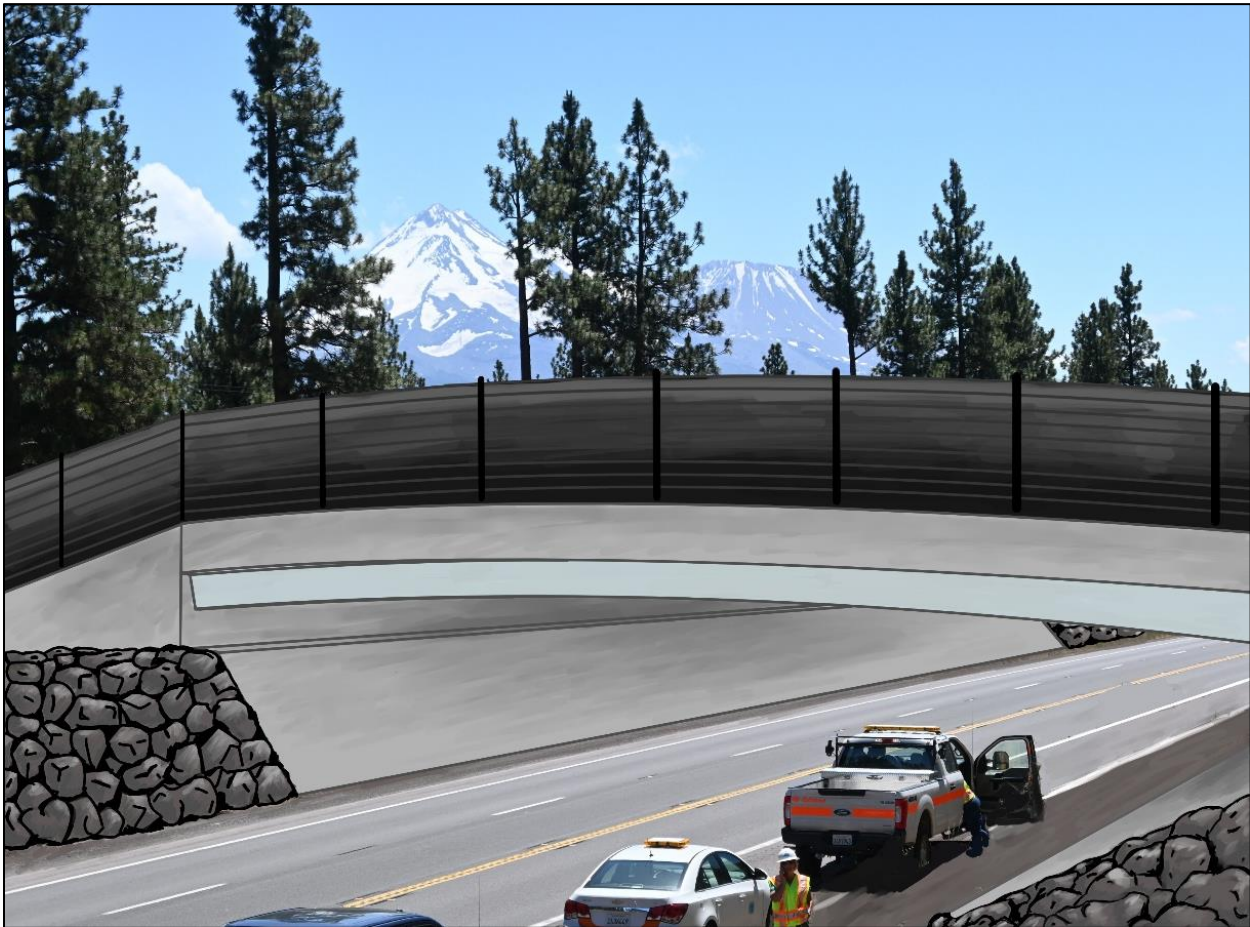
Figure 40: Rendering of US-97 FRP wildlife overpass with Mt. Shasta in the background.
