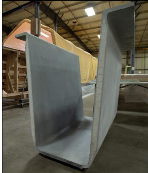
Figure 22: A section of a CT Girder made by AIT. Foam inserts can be seen in the vertical walls of the girder to help reduce the weight (Francis, 2019).
