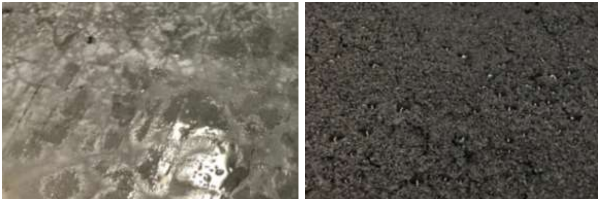
Figure 78. Images of NaCl solution application on (left) concrete and (right) asphalt samples.
