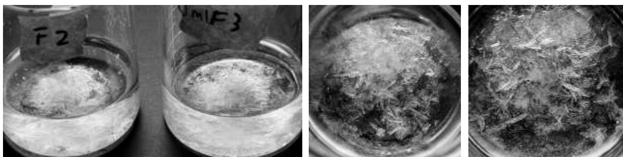
Significant ice crystal formation and salt precipitation for solution F2 and F3 (left), close-up images of F2 (middle) and F3 (right) at -6^{\circ}\text{F}
