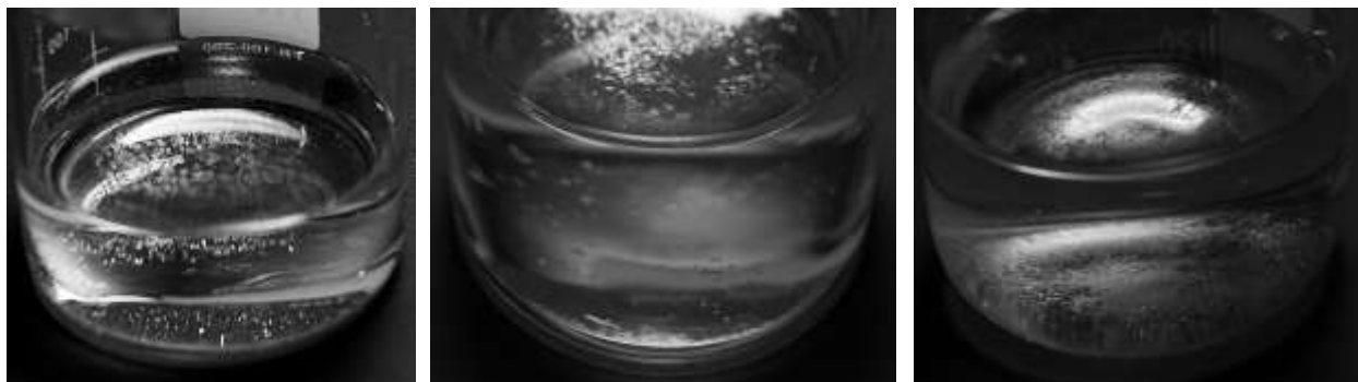
Ice crystal formation and salt precipitation at 5°F for E triplicates (E1 to E3: left to right)
