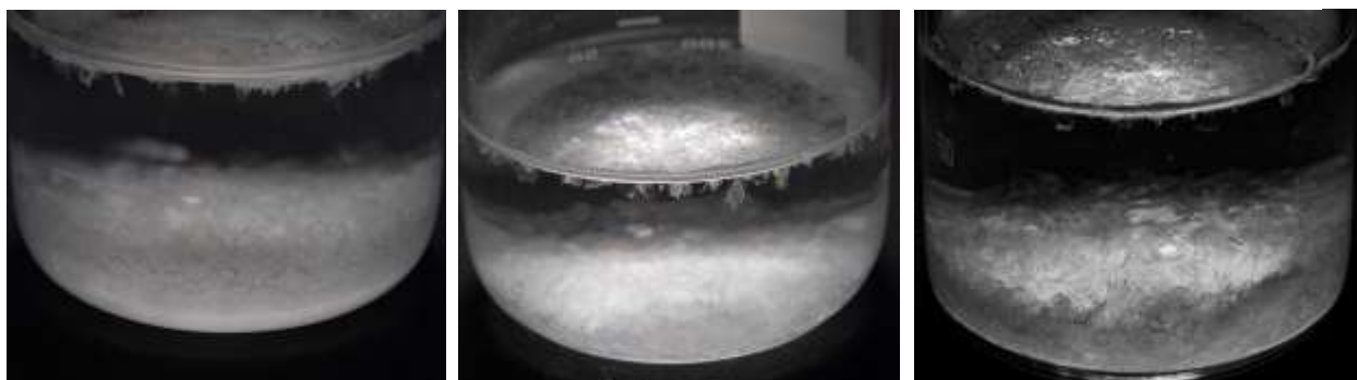
Ice crystal formation and salt precipitation at 5°F for H triplicates (H1 to H3: left to right)
