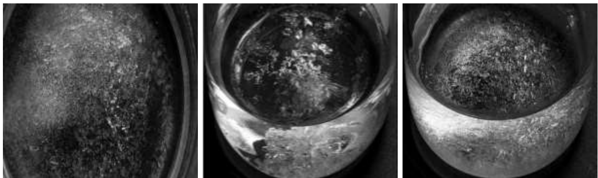
Significant ice crystal formation and minor salt precipitation at 0°F for F triplicates (1 to 3: L to R)
