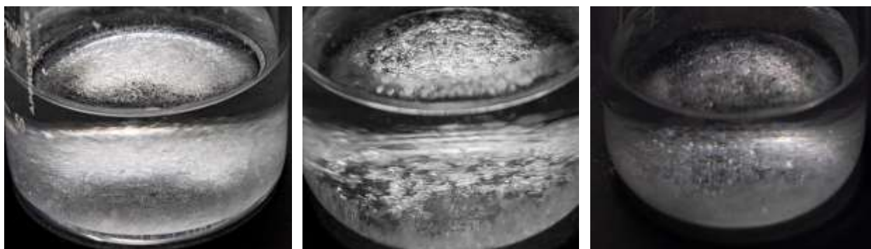
Ice crystal formation and salt precipitation at 5°F for F triplicates (F1 to F3: left to right)
