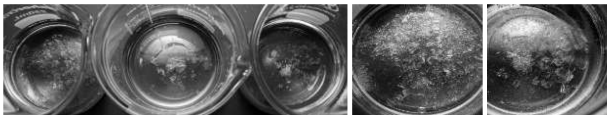
Significant ice crystal formation and salt precipitation for solution E triplicates (left), E1 (middle), E3 (right) at -6^{\circ}\text{F}
