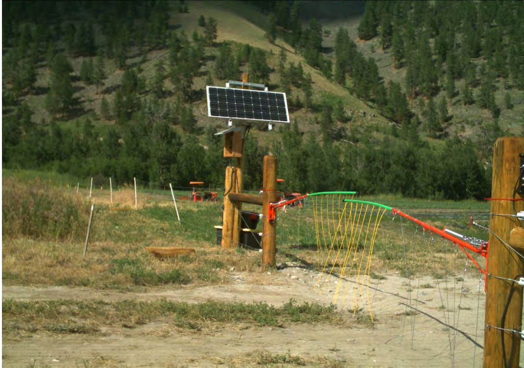
Figure 6: A drive-through bump gate (not modified) (about 16' (4.88 m) wide, about 3' (91 cm) tall), with vertical electrified wires. The orange horizontal pole is metal and carries current. The green horizontal part is fiberglass and does not carry current.
