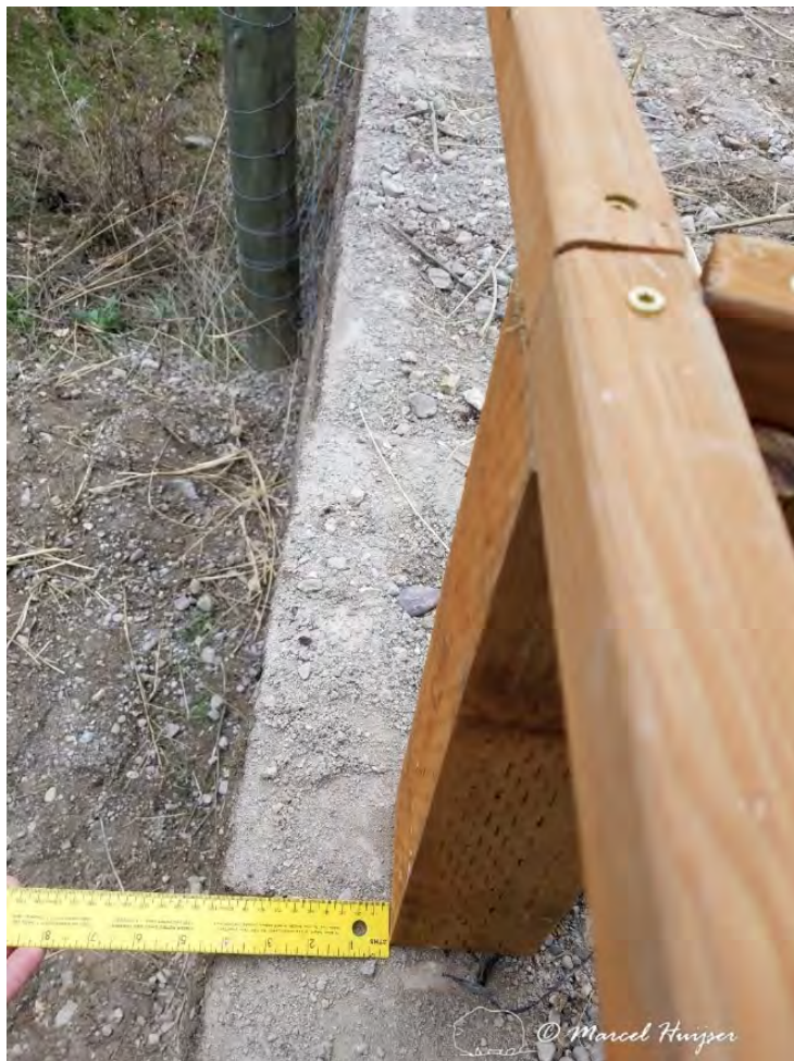
Figure 10: The wooden prototype had a setback of 4 inches (10 cm).
