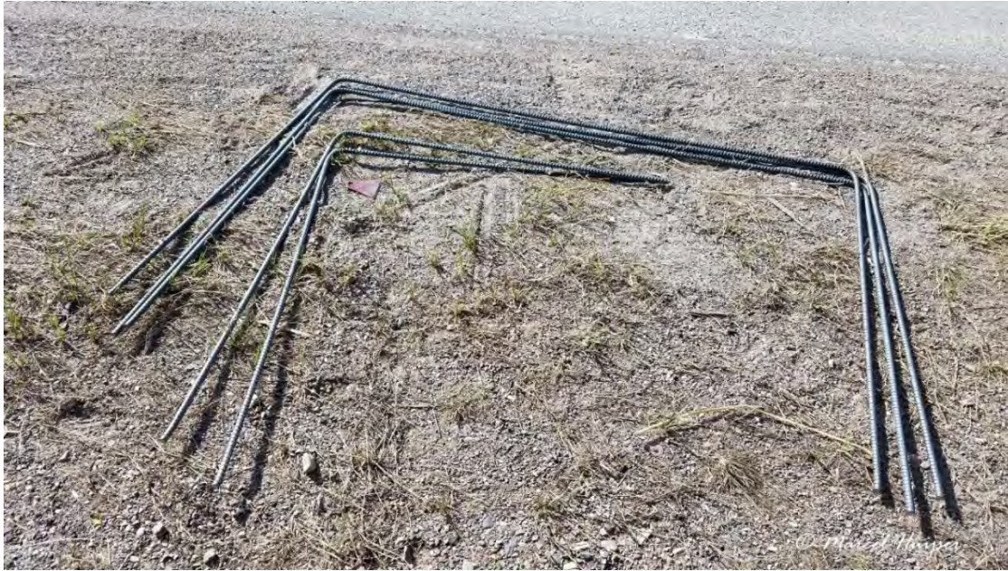
Figure 6: Several of the “staples” (60-inch horizontal, 42-inch legs) the L-shaped corner elements (36-inch swing arms, 42-inch legs).
