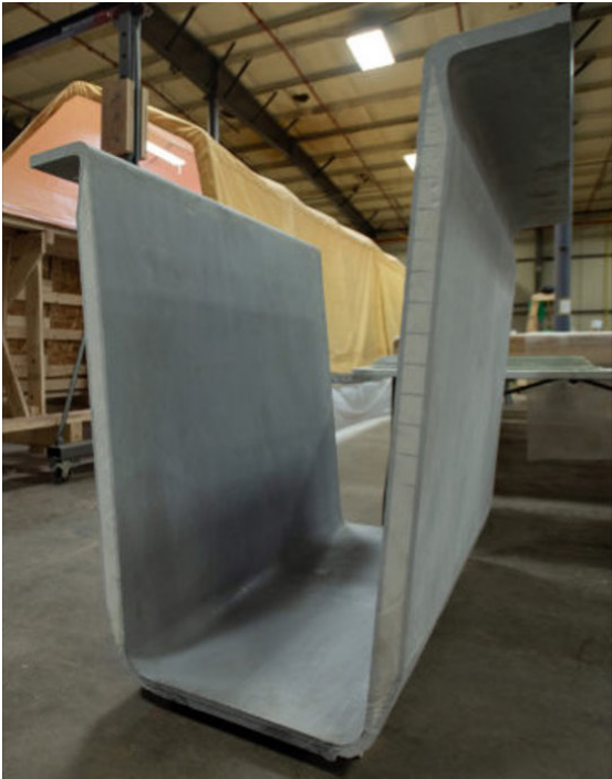
Figure 17: A photo and the dimensions in centimeters (cm) of the FRP or composite tub girder used to form the structure for the design of the wildlife overpass structure on US-97 in Siskiyou County, California (AIT Bridges). Not drawn to scale
