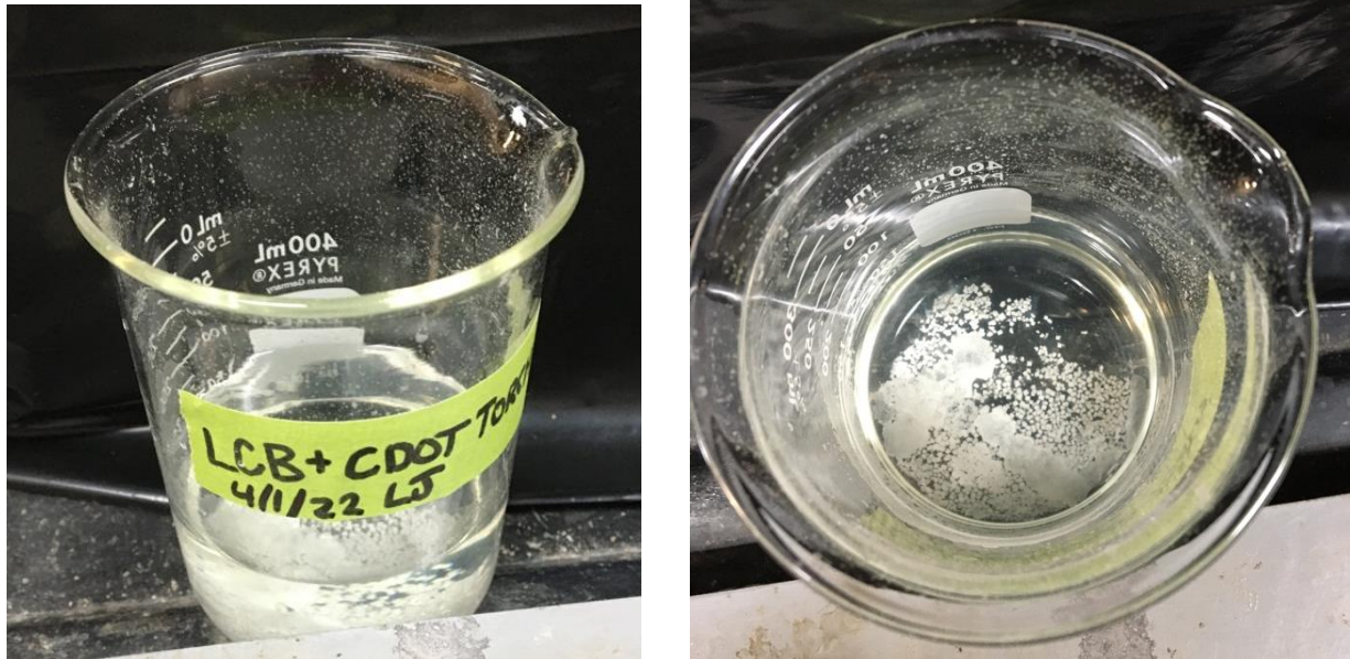
Figure 2. Photographs of 6% Torch by volume added to LCB1 showing precipitate present at the bottom of the beaker.
