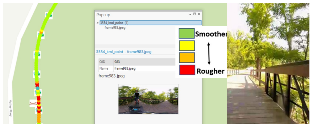
Photographic, annotative and accelerometer data layered together in ArcGIS. 360-degree photographs viewed within ArcGIS
