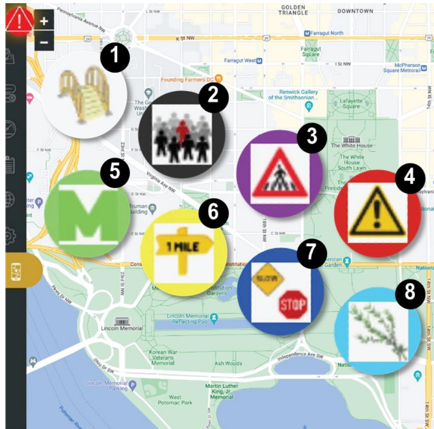
Figure 14: Smart Delta user interface with map and annotations. The numbered icons are: 1) bridge, 2) congestion, 3) crosswalk, 4) hazard, 5) trail surface material change, 6) milepost, 7) slow/stop, and 8) vegetation.
