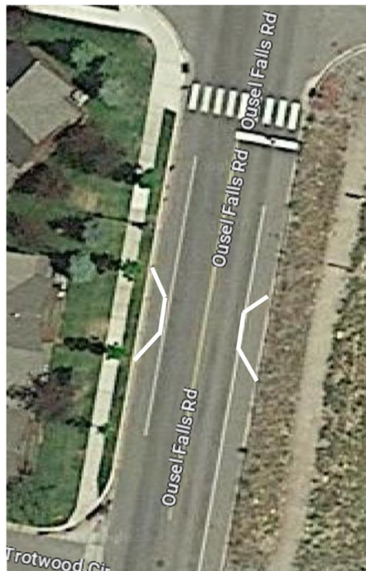
Figure B-4: Gateway curb extension on Ousel Falls Road.
