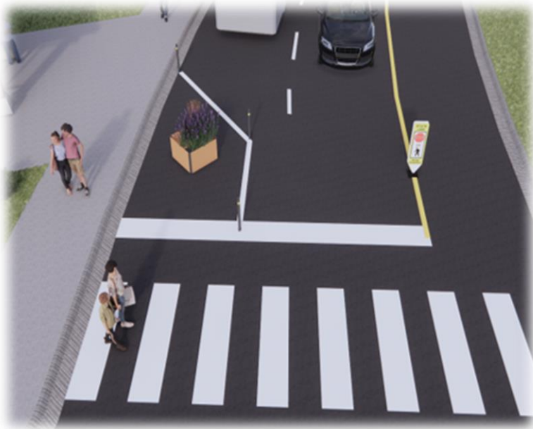
Figure 6. A sketch of a curb extension that decreases the overall width of the roadway for pedestrians.
