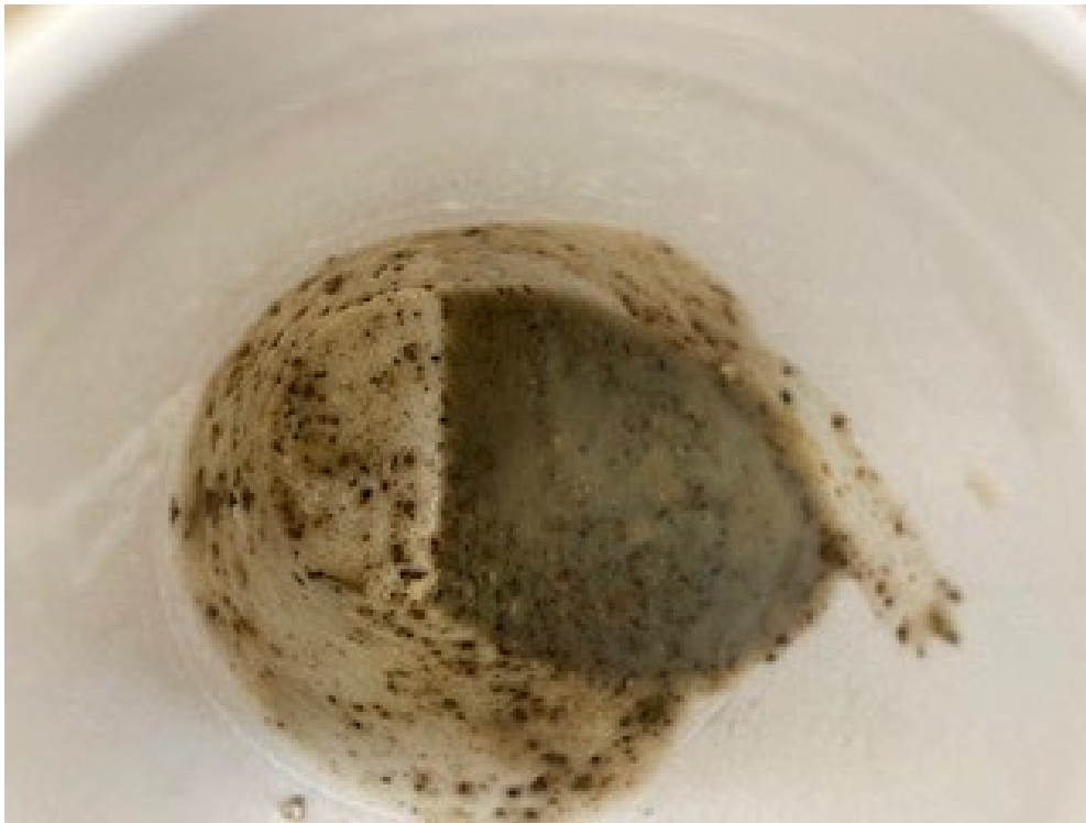
Figure 3. Off-white thick scum that clogged the flow meter and nozzles of the liquid application system.
