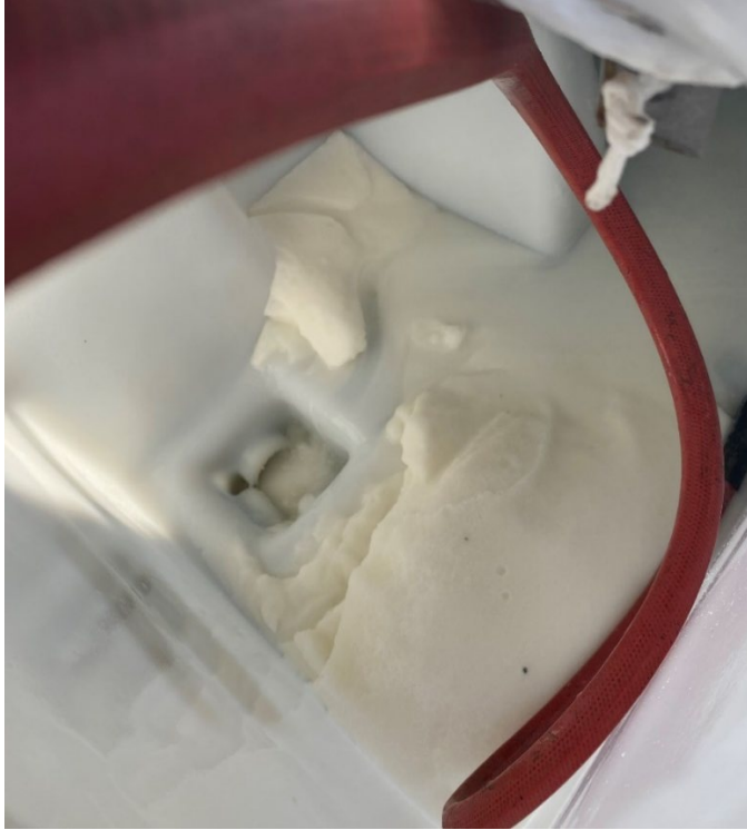
Figure 7. Tank with solid salt precipitated out at the bottom of the tank.
