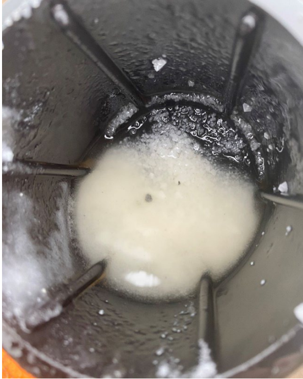
Figure 5. Truck filter clogged with solid salt crystals.
