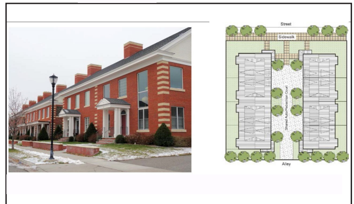
Figure 38.520.040.C.2.a. Direct pathways between the street and dwelling units are required. Photo Source: City of Bozeman
