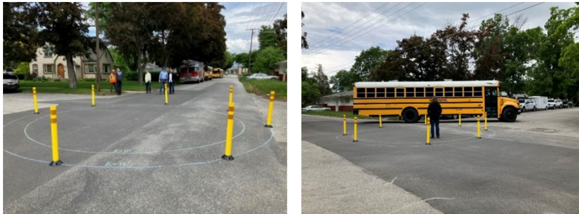
Figure 2: 12- and 10-foot radius circles were drawn in chalk at the S. 3 rd & Baker intersection to test large vehicle turning movements (left), including school buses (right).
